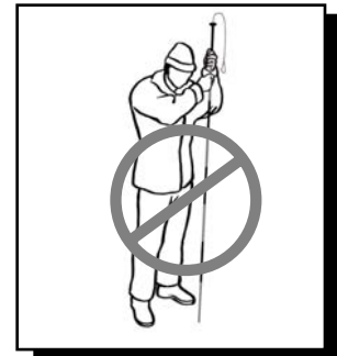
Figure 2: Incorrect probe technique
